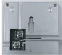
**Step 5.** Integrate the remote temperature sensor with the screws as the order of arrows.
