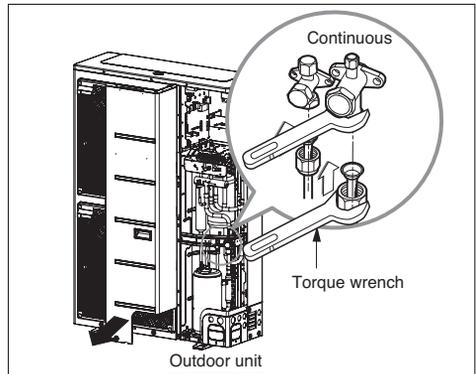
※ When tighten the pipe, hold the hexagonal body.
