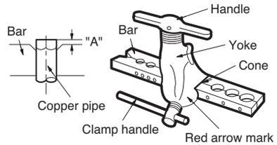
Firmly hold copper tube in a bar(or die) as indicated dimension in the table above.
